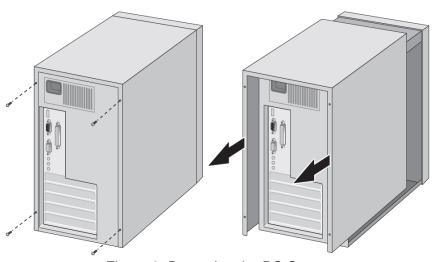
Figure 3. Removing the PC Cover
